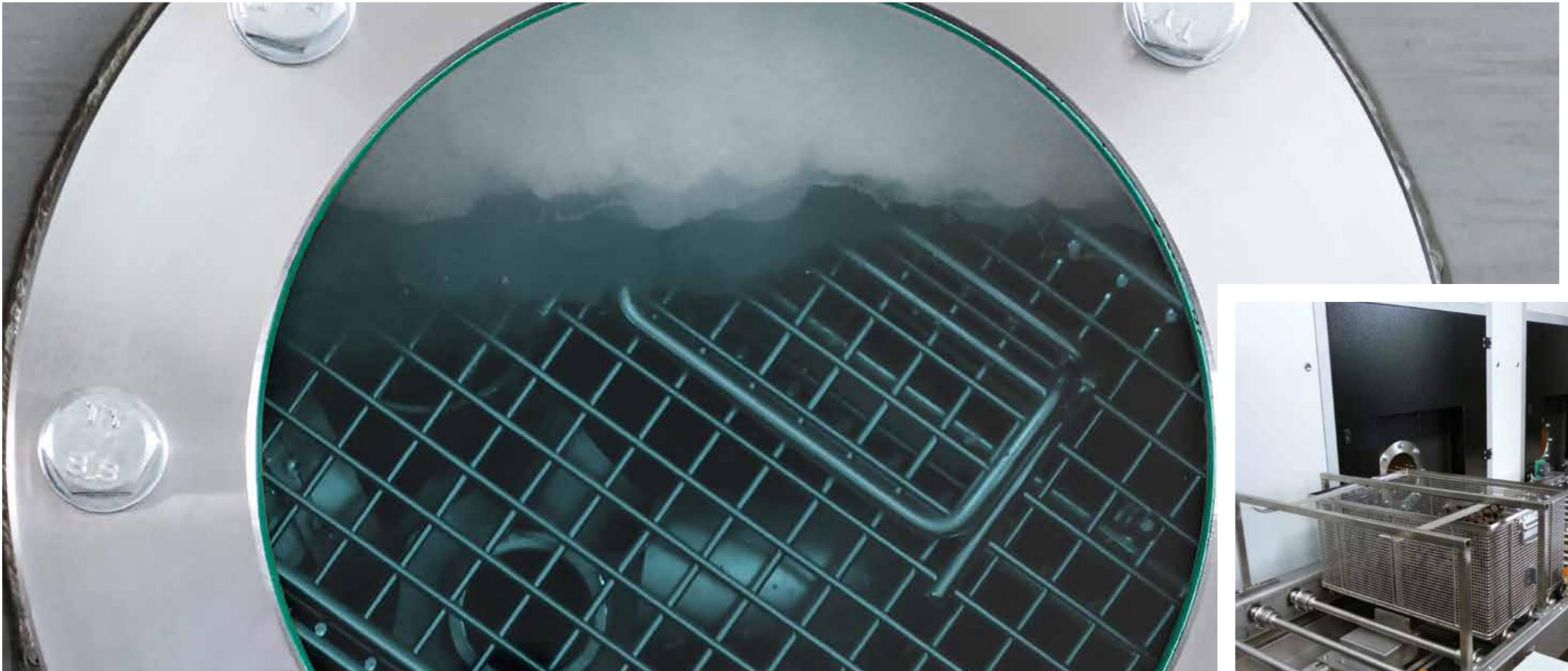
After the TEM process, the burnt material deposits in the form of ferric oxide on the whole surface of the workpiece. Due to this fact, a subsequent treatment of the components is generally necessary. Exceptions exist for workpieces which are subsequently subjected to galvanization, nitration or hardening.
